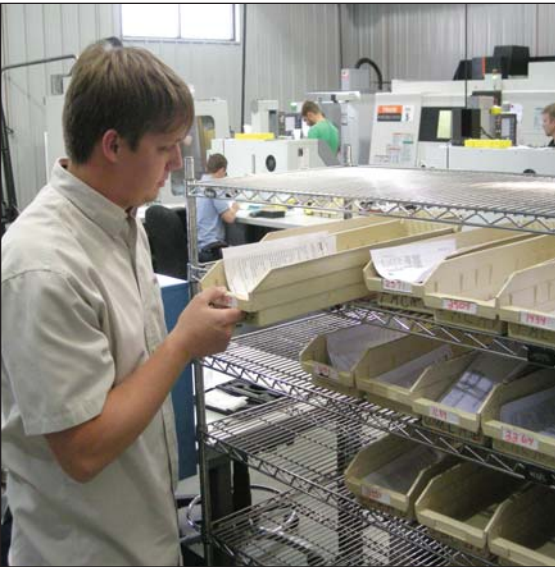
Machine Shop Manager Brent Bowden shows the “fifo” lane implemented to ensure that parts are processed on a first-in-first-out basis to help ensure efficiency and timely delivery.
