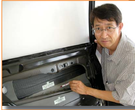
Below: Seoil-America Management Director Jerry Chang shows how the firm's product is used in automobile doors as a vibration dampening medium.
